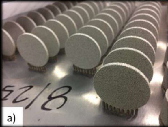
a) Typical layout for testing a variety of parameters settings on standard discs.
