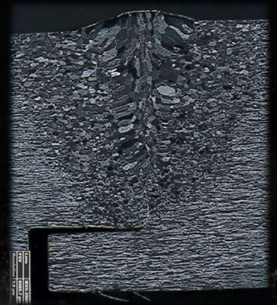
Example precision Molybdenum-Molybdenum weld
