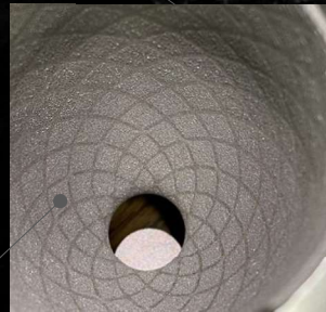
DurAMesh Porosity Incorporated into a Chamber Design
