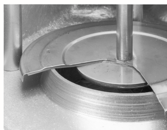
Cutaway of Air-Cushioned Pallet Assembly
